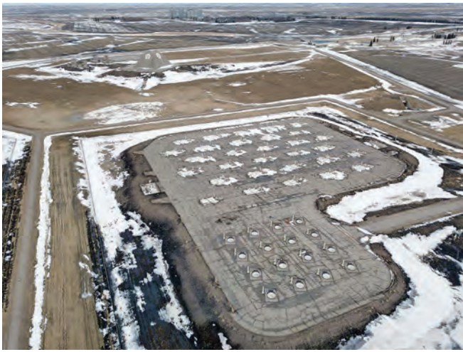
Drone photograph of the Missile Support area. 16x Sprint silos in foreground with 30x Spartan silos to rear. Photo Chris Howells
